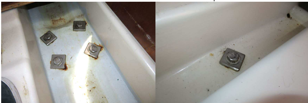
Keel bolts without corrosion
