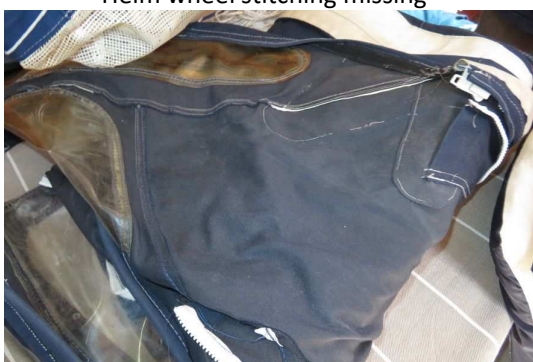
Sprayhood stitching repairs failed
