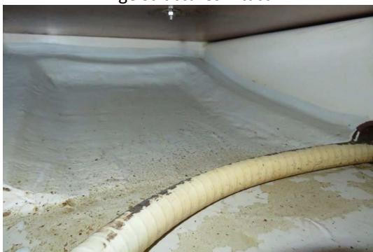
No separation of liner and hull
