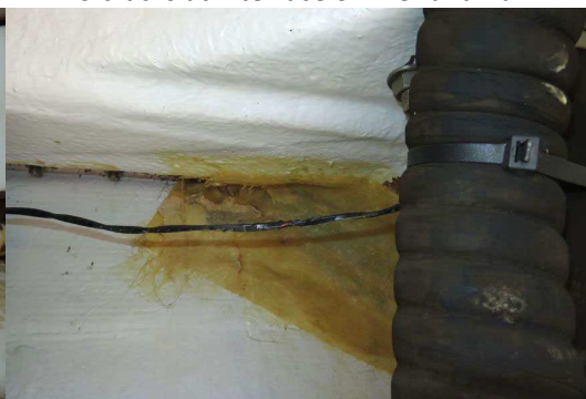
Fiberglass repairs under stern cleats
