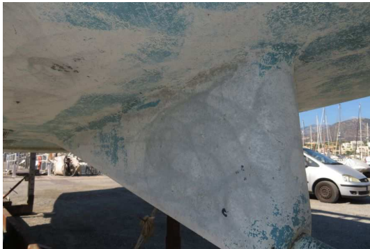
Skeg secure to the hull
