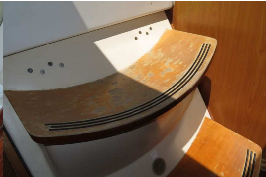
Typical deterioration to varnish at companionway
