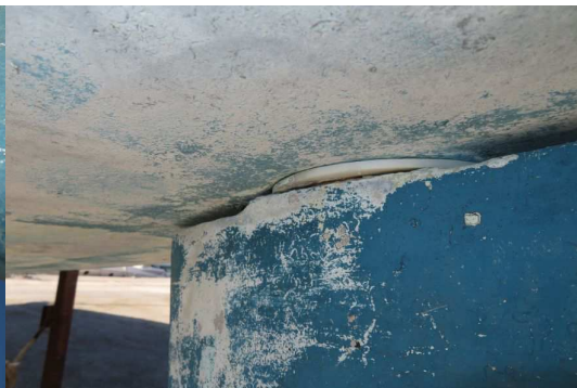
No cracks near rudder post
