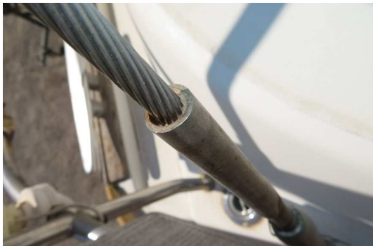
No broken wires at entry to swage terminals
