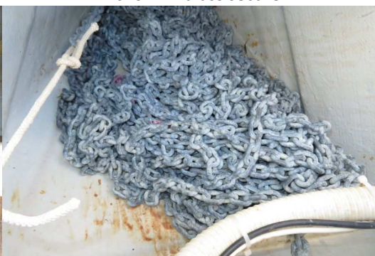
Chain with galvanising intact
