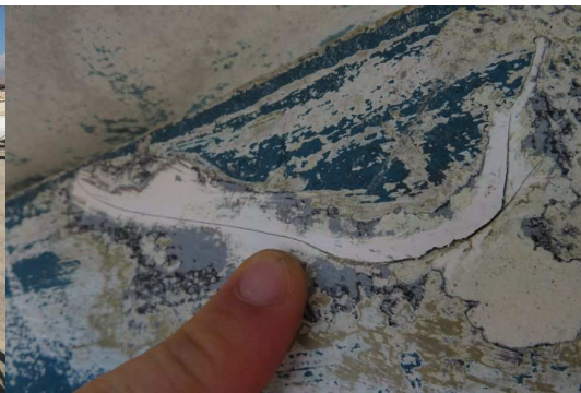
Gelcoat crack to rudder
