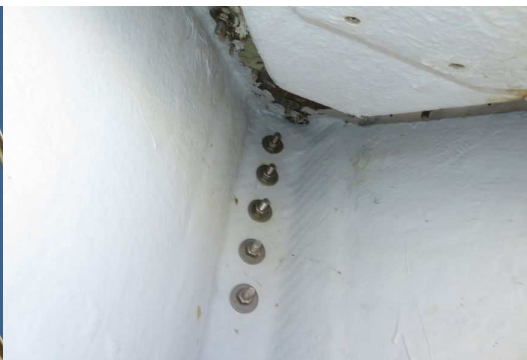
Stemhead bolts without corrosion
