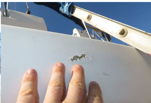
Small gelcoat repair required at stern
