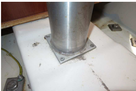
No damages at compression post step
