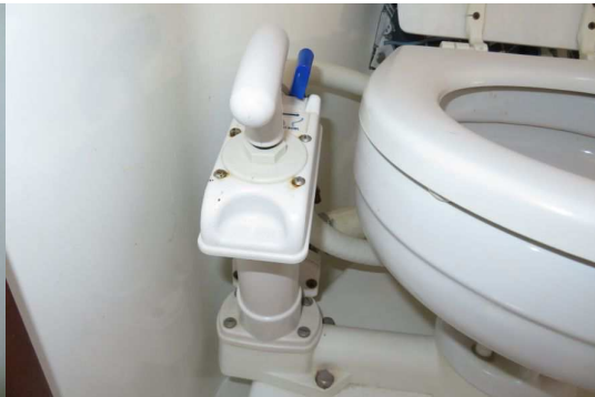
Manual pump no sign of leak
