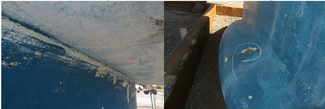
Hull to keel join was tight
