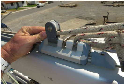
Outhaul requires replacement. Sheave block chipped
