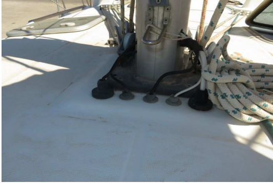
No compression or cracks at mast deck step
