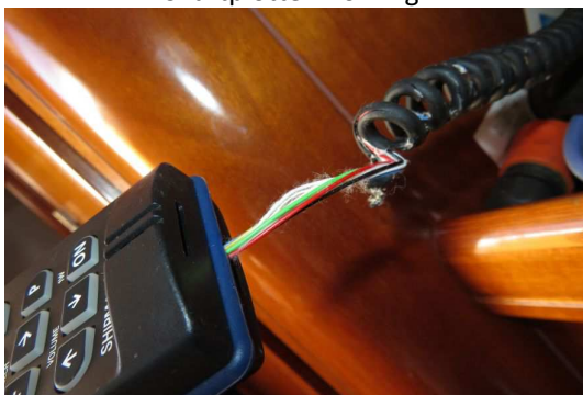
VHF cable damaged
