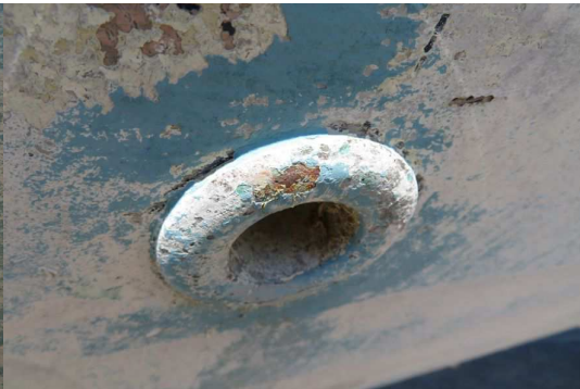
Through hull neck without wastage
