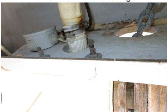
Anchor windlass bolts without corrosion
