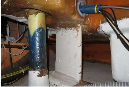
Rudder tube secure
