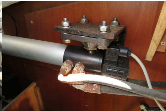
Connections at cylinder corroded
