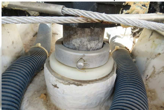
Rudder tube top without crack
