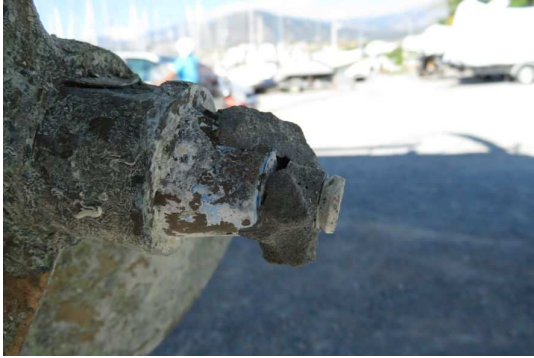
Propeller nut anode fully wasted
