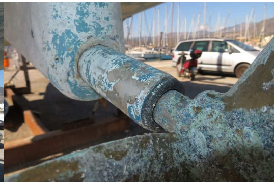
No excessive play at cutlass bearing
