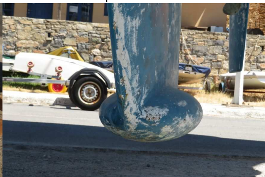
No damages at leading edge
