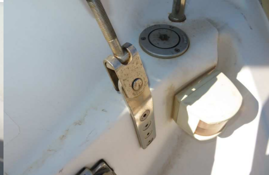
No crazing around backstay chainplates
