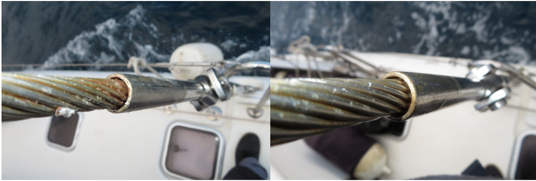
Shroud lower swages without broken wire
