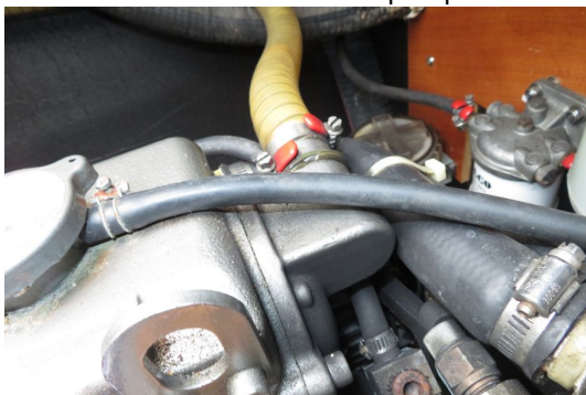
No leaks at heat exchanger ends
