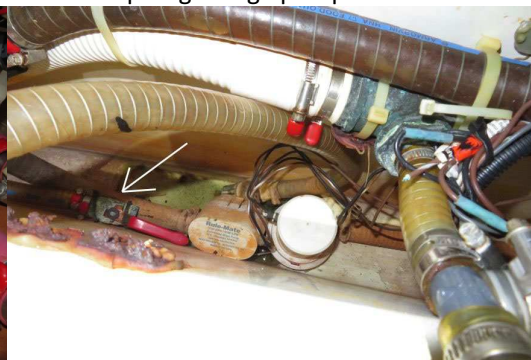
Drain hose fallen into bilge where the valve cannot be closed
