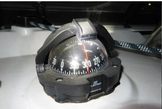
Magnetic compass no bubble
