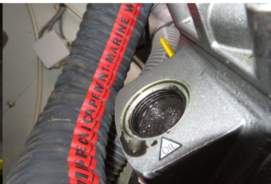
Oil without sign of water contamination
