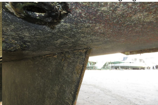
No cracks to hull around trailing edge
