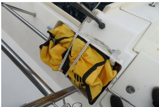
Rescue sling missing cover to box
