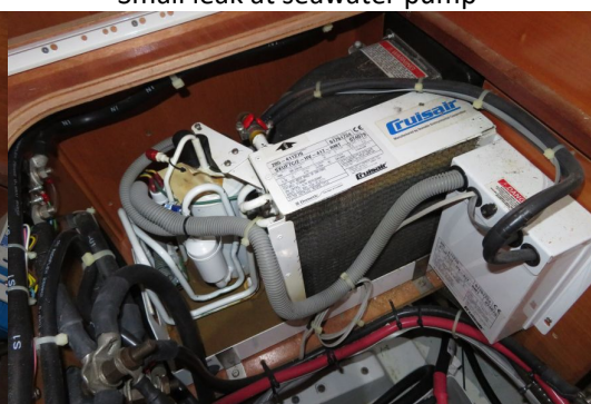
Air handler without corrosion
