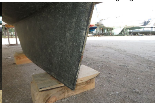
No damages at trailing edge
