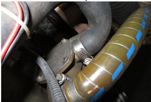
No leaks at seawater pump
