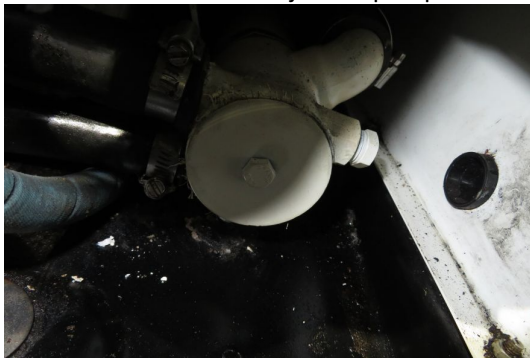
Only minor leak at heat exchanger
