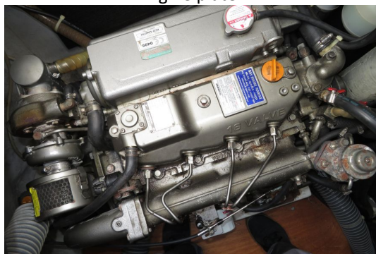
Engine with minor corrosion
