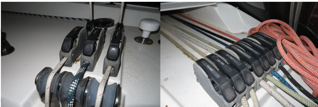
Rope jammers without damages
