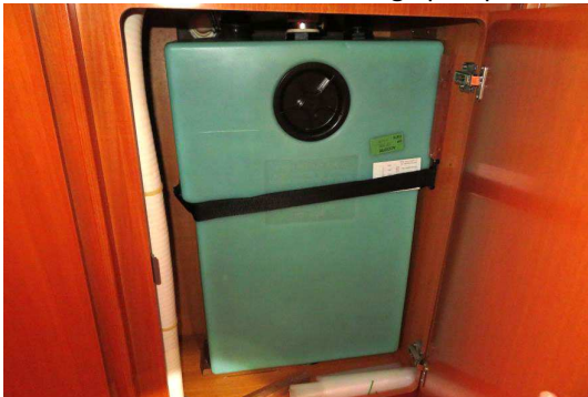
No leaks at owners holding tank
