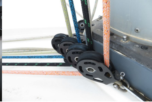
Sheaves without deterioration
