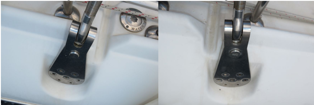
No gelcoat crazing around shroud chainplates
