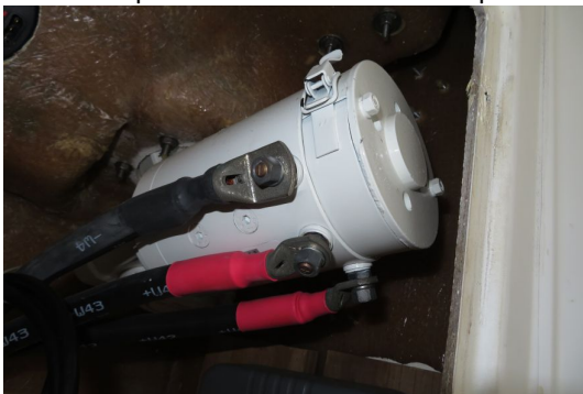
Winch motor without corrosion
