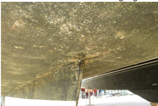
No cracks to hull around trailing edge
