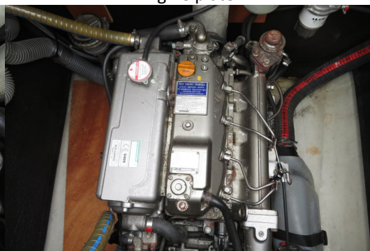
Engine with minor corrosion
