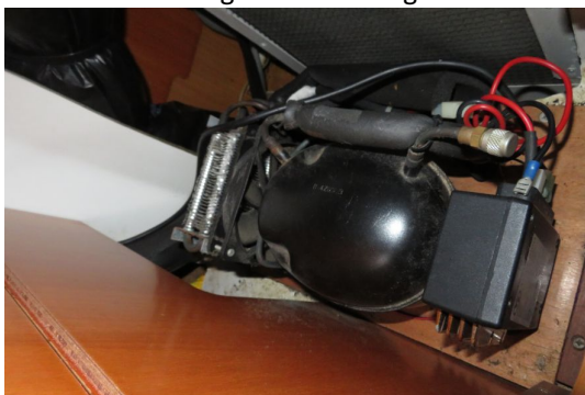
Compressor with coatings intact
