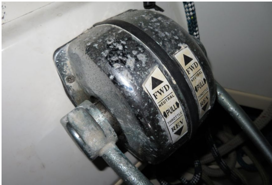
Engine controls with cosmetic deterioration of the chrome plating
