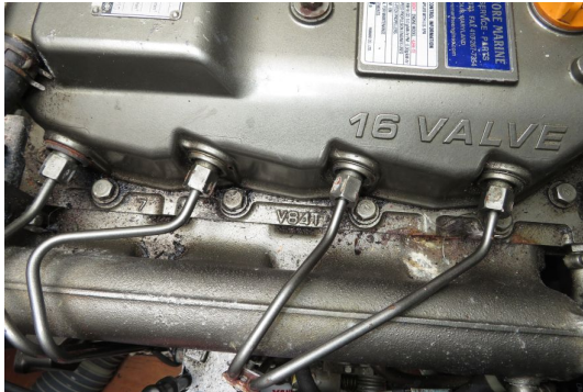
No leaks at injectors
