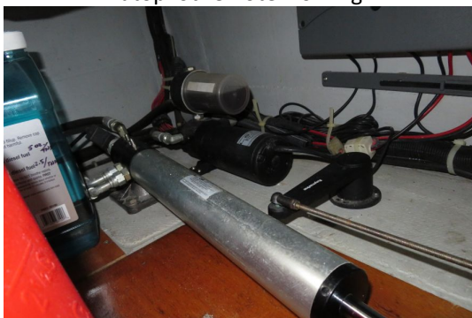
No leaks at hydraulic autopilot
