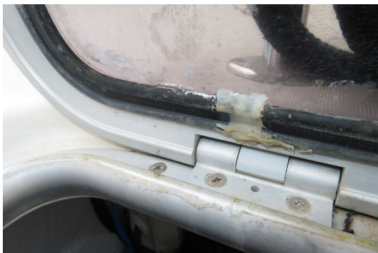
Hatch seal requires replacement not this temporary repair
