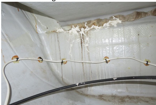
Sealant applied at stern minor leak
