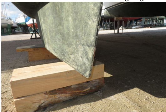
No damages at trailing edge
