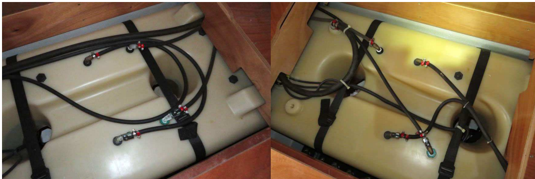
Fuel tank no leaks from connections
