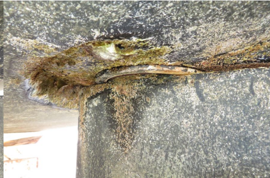
No cracks at top of rudder
