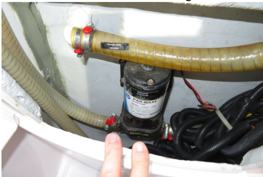
No leaks at toilet flushing water pump
