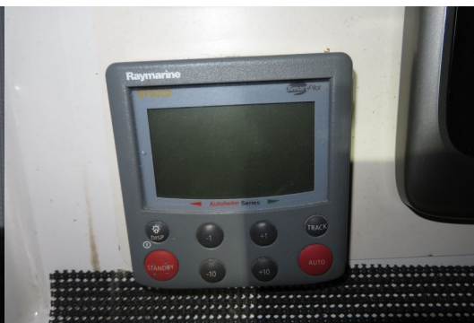
Autopilot control not working
