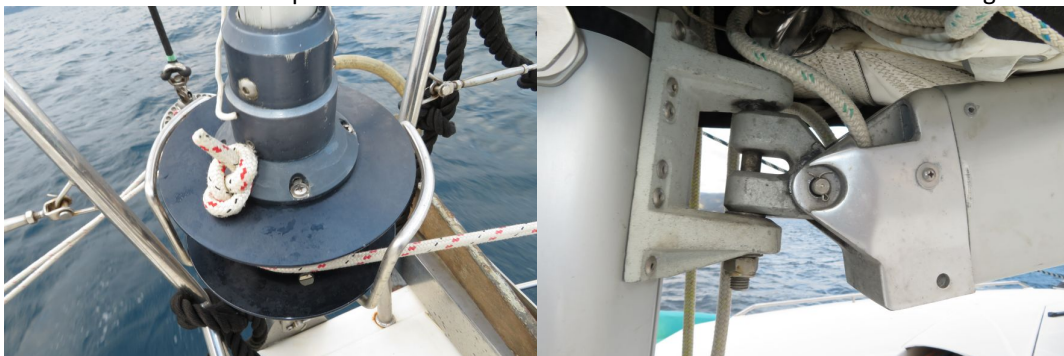
Furler drum intact and with free movement
