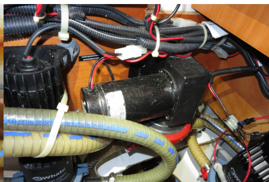
Diaphragm bilge pump no leaks
