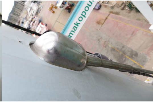
Diamond upper swages without broken wire
