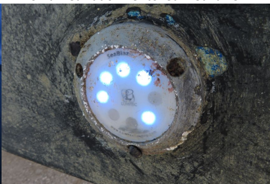
Starboard underwater light partly failed
