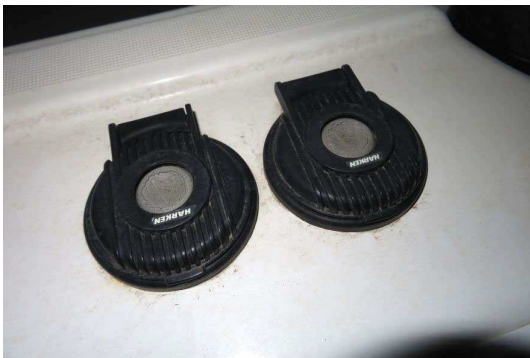
Aft cockpit winch footswitches to replace
