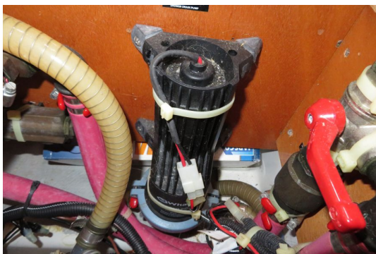
Grey water pump no leaks
