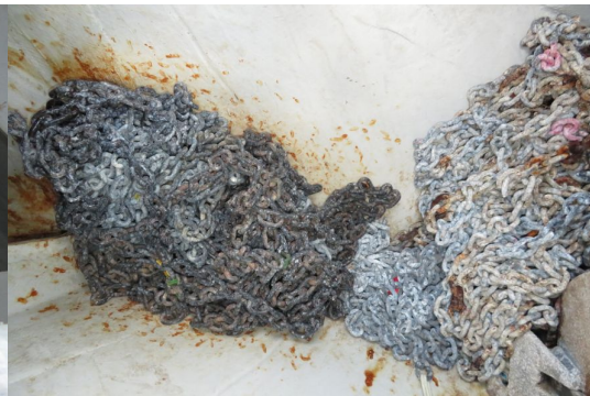
Chain with galvanising reasonably intact
