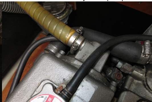
No leaks at heat exchanger ends
