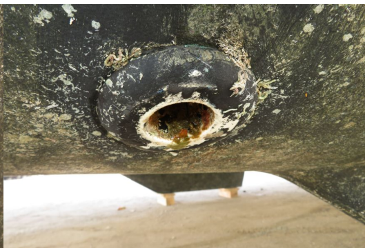
Plastic through hull without cracks
