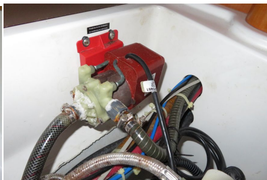
Small leak at seawater pump
