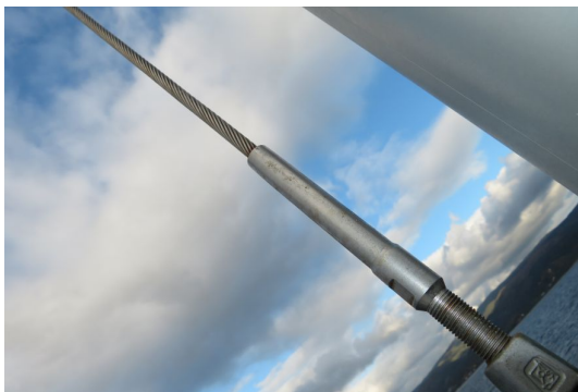
Diamond lower swages without broken wire
