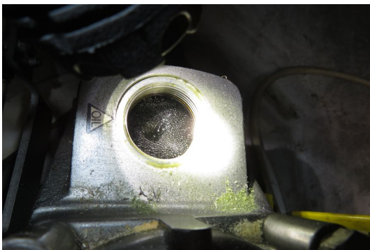
Oil without sign of water contamination
