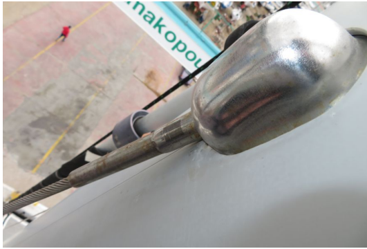
Diamond upper swages without broken wire
