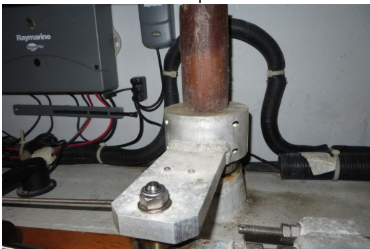
Steering gear without corrosion
