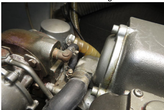
No leaks at heat exchanger ends
