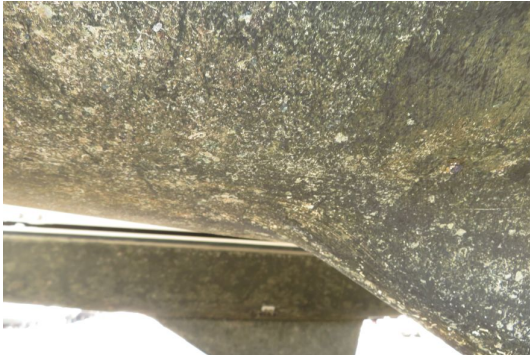
No cracks to hull around leading edge
