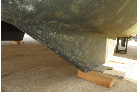
No damages to hull at leading edge
