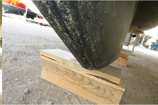
No damages to hull at leading edge
