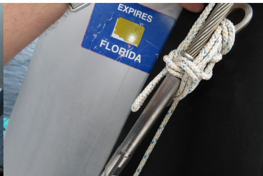
Diamond lower swages without broken wire
