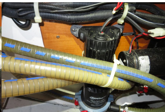
Grey water pump no leaks
