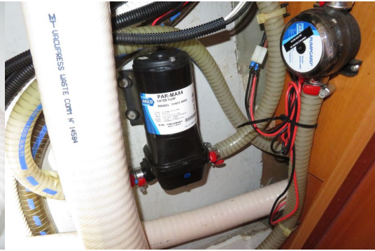
No leaks at toilet flushing water pump
