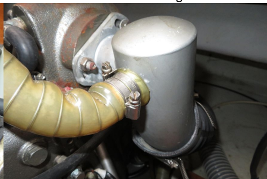
No leaks at exhaust mixing elbow
