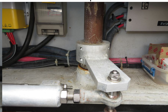
Steering gear without corrosion
