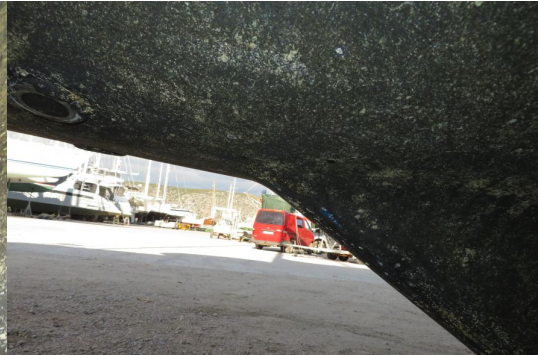
No cracks to hull around leading edge
