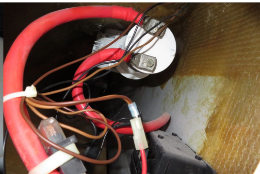
Winch motor without corrosion
