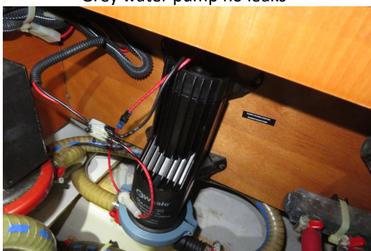
Grey water pump no leaks
