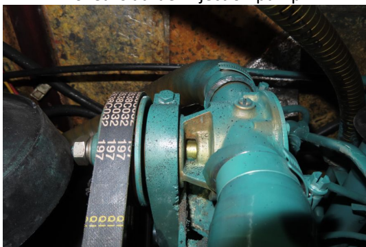
No leaks at seawater pump
