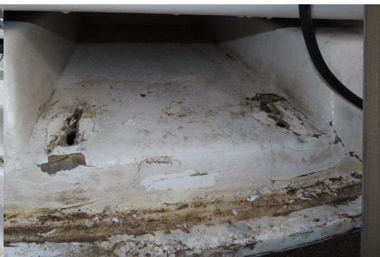
Repairs required to holes at bathing ladder
