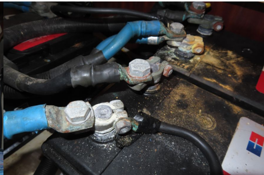
Sulphation at battery terminal
