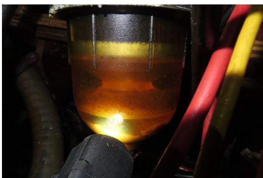
Primary fuel filter with sediment
