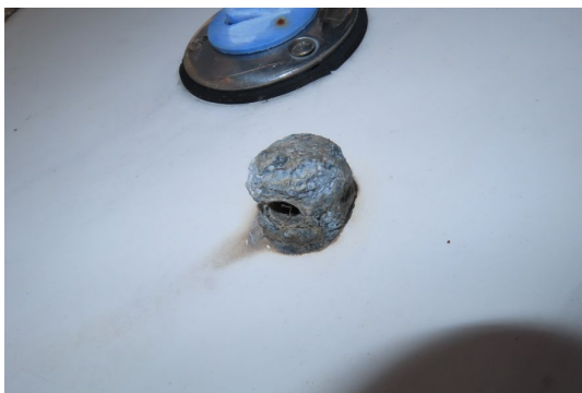
Corroded tank vent
