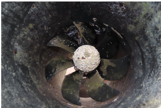
Bow thruster propeller without damage
