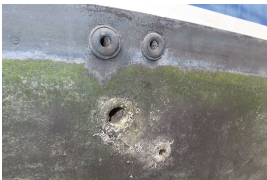
Through hull fittings without wastage
