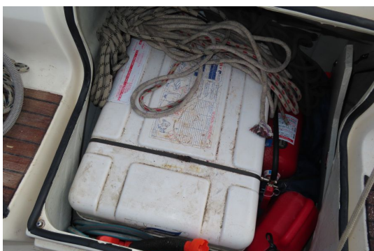
Liferaft casing was intact
