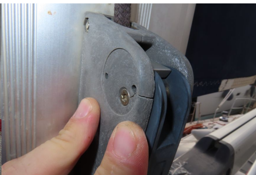
Cracked rope jammer
