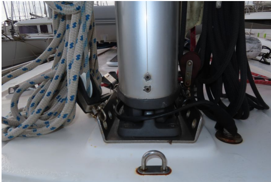
No cracks or compression at mast deck step
