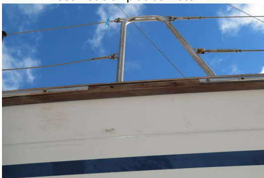
Missing stainless rubbing strake
