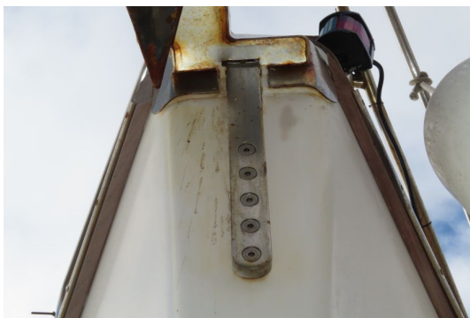
No corrosion at stemhead fitting
