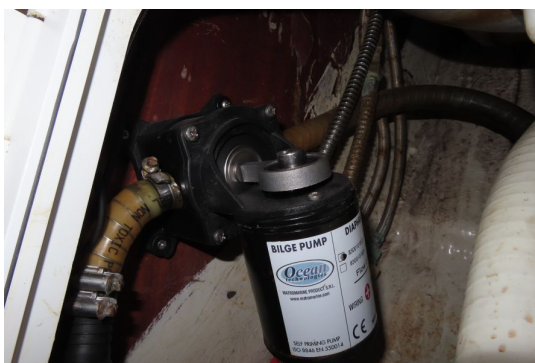
Shower drain pump no leaks
