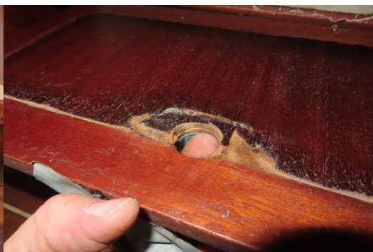
Wet damage at galley
