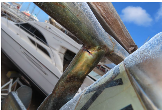
Pulpit framing cracked
