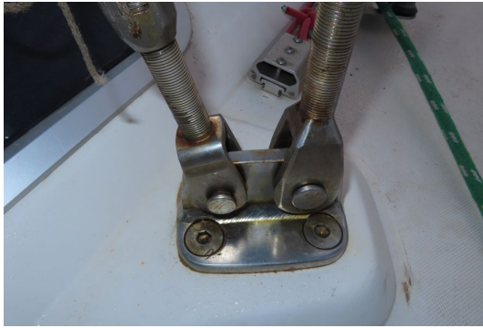
No cracks at shroud deckplates
