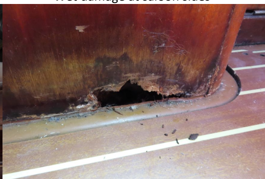
Wet damage at aft port heads exterior
