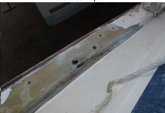
Repairs to hull to deck join
