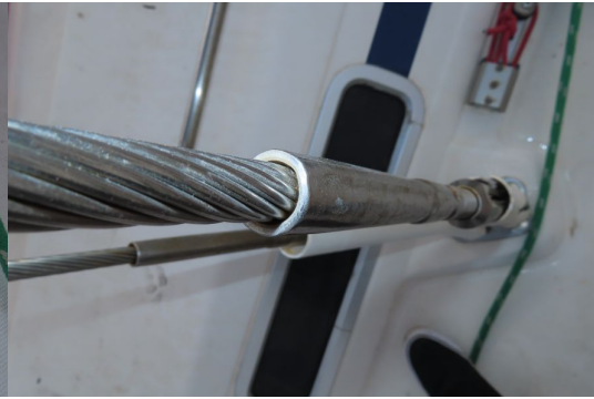
No broken wires
