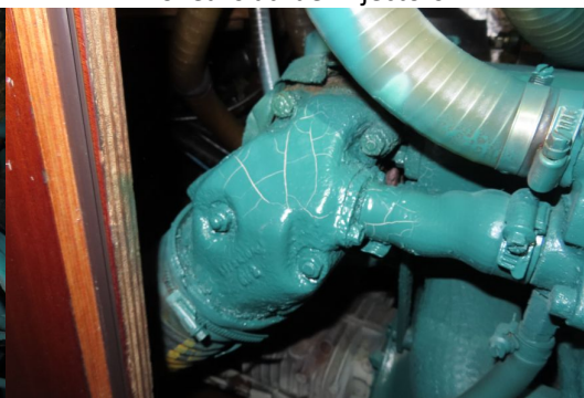
No leaks at exhaust elbow
