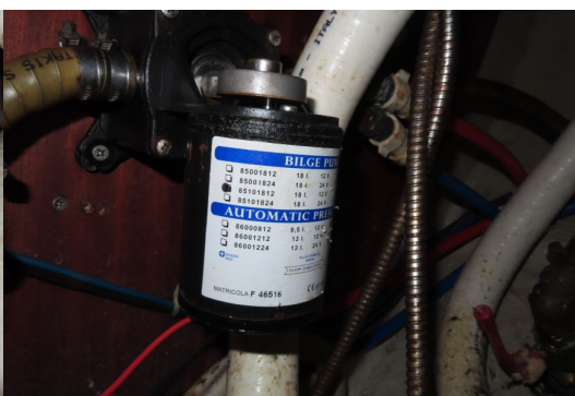
Shower drain pump no leaks
