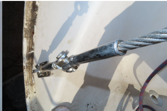
Backstay no broken wires
