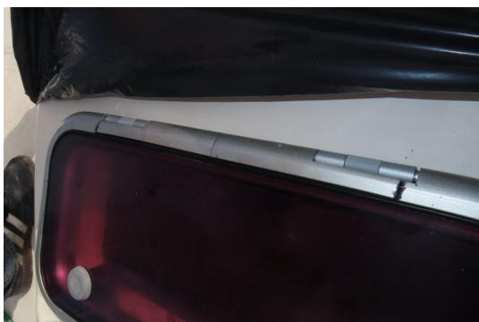
Frame of hatch window separating
