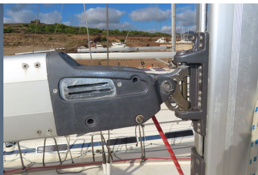
Boom gooseneck without fracture
