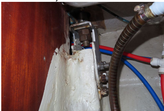
Shroud chainplates were secure
