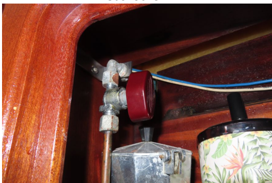
Shut off valve without corrosion
