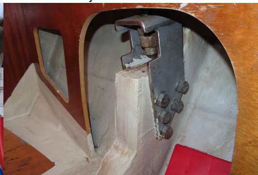
Shroud chainplates were secure
