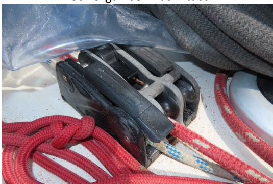
Missing handles of rope jammer
