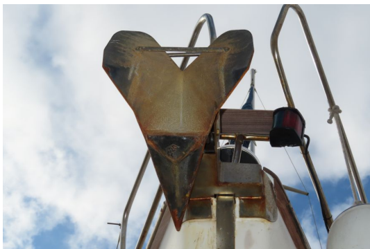
Anchor with minor corrosion
