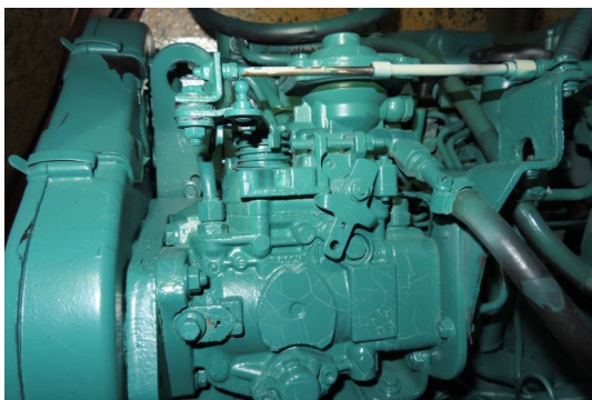
No leaks at fuel injection pump
