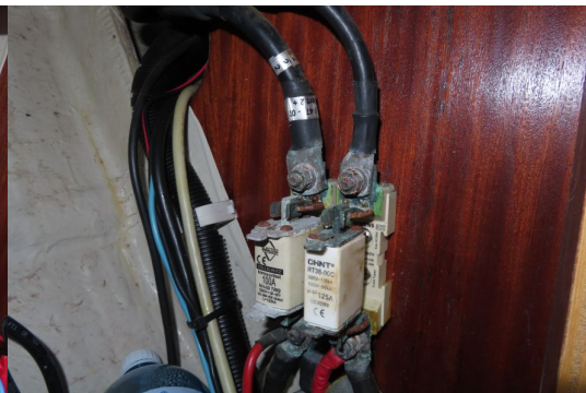
Electrics with corrosion
