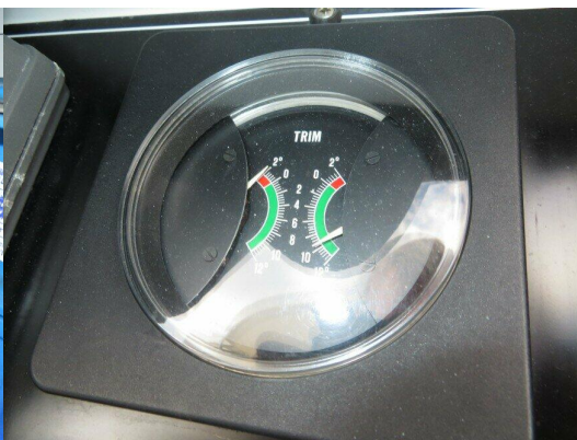
Port flybridge trim tabs angle indicator does not work properly
