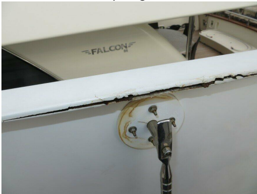
Hatch to flybridge requires fibreglass repairs
