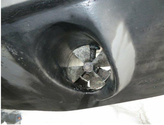
Bow thruster tunnel secure to hull
