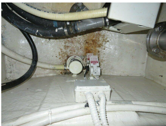
Submersible bilge pump and high level alarm
