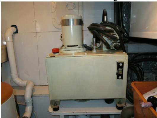
Steering hydraulic power pack no leaks
