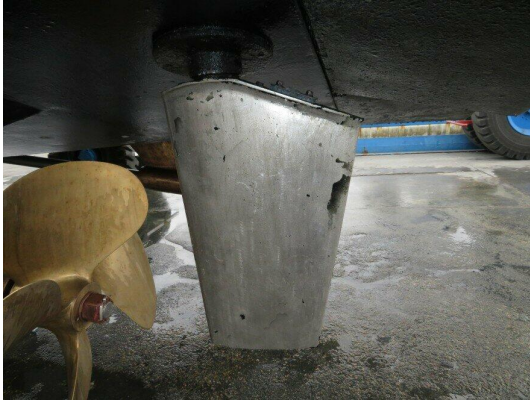
Port rudder without wastage
