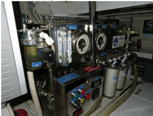
Watermaker without corrosion or leaks
