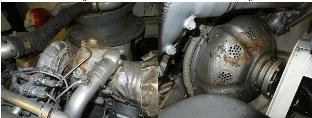
Engines some small corrosion areas
