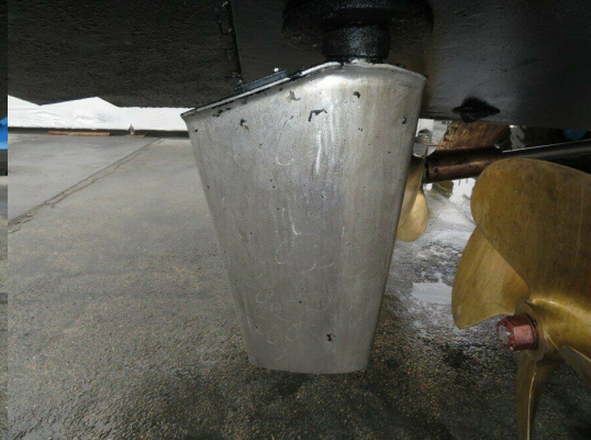
Starboard rudder without wastage
