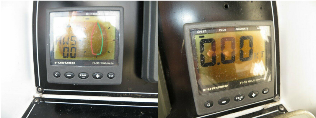
Flybridge small instruments with sun damage Flybridge small instruments with sun damage
