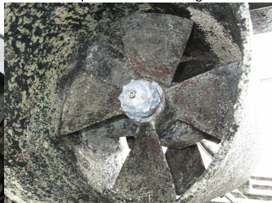
Stern thruster propellers without damage
