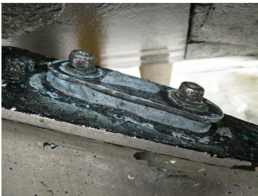
Rudder anodes suitable for further use
