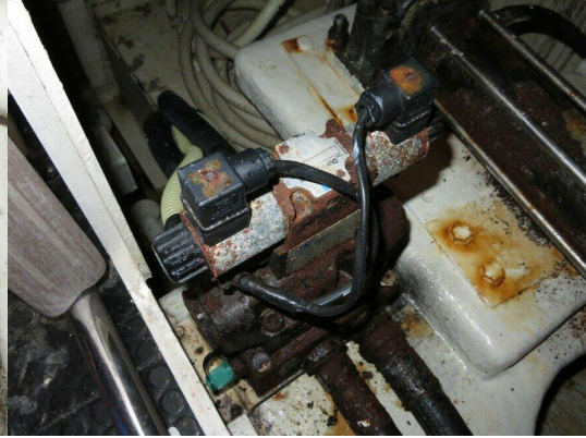
Trim tabs electronic valves with corrosion
