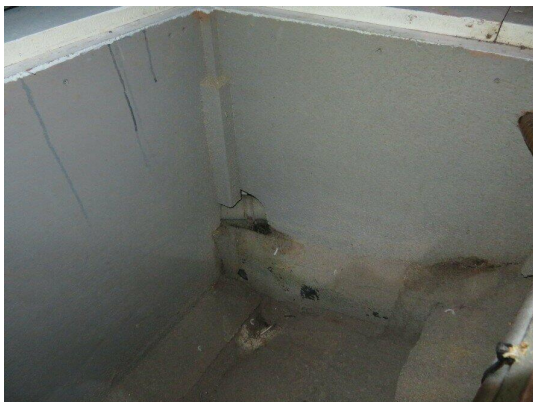
Bilge with spray foam insulation
