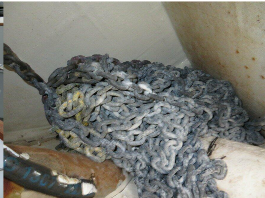
Chains with galvanising intact
