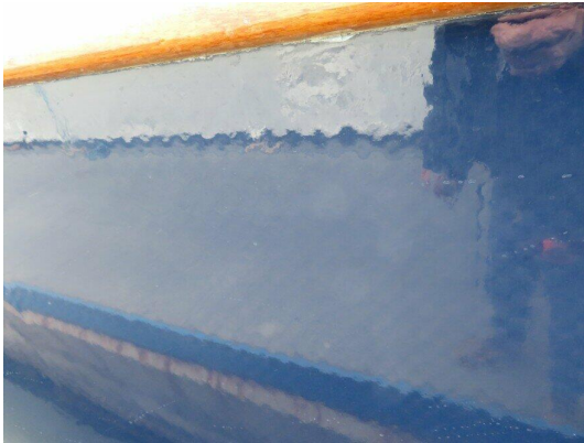
Poor topside fairing under the paint with the laminate weave clearly visible (poor)
