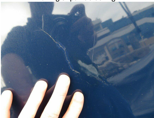
Fairing of paint cracking
