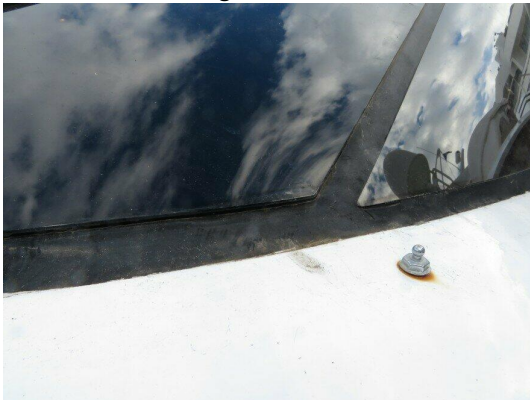
Wheelhouse window seals not deteriorated
