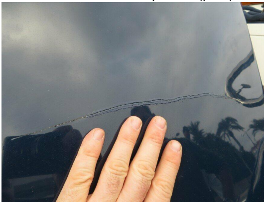
Fairing of paint cracking
