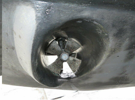
Bow thruster tunnel secure to hull
