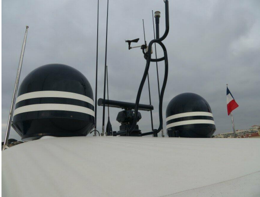
Radar arch equipment coatings intact
